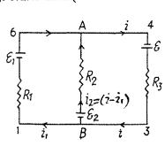
3.183 Indicate the currents in all the branches using charge conservation as shown in the figure. Applying loop rule,  $-\Delta \varphi = 0$  in the loops 1A781, 1B681 and B456B, respectively, we get
