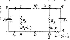
3.184 Indicate the currents in all the branches using charge conservation as shown in the figure. Applying the loop rule  $(-\Delta \varphi = 0)$  in the loops
